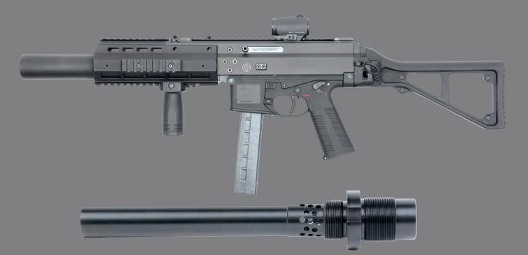
The holes in the barrel, directly in front of the chamber of the APC9-SD, reduce the pressure of the propelling gases. So normal supersonic ammunition is slowed down to subsonic speed. No expensive subsonic ammunition needed.
