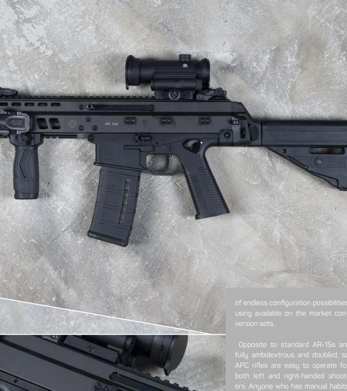
Charging handle can be easily moved to the other side of APC556/APC223 without any tools. To change the side, simply pull the bolt carrier to the rear and slide the handle. Case ejection port is fixed and cannot be changed to the other side, but left-handed shooters should not have any problem because cases are ejected almost perpendicular to the weapon axis.
