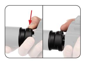
b. Remove the suppressor from the 3-lug.
