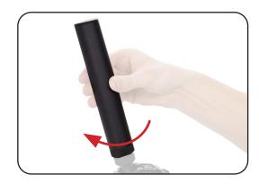
h. Checking: If the suppressor is mounted correctly, it cannot be slid off the 3-lug by pulling on it.
