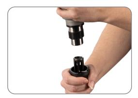
c. Remove the nut from the barrel.
