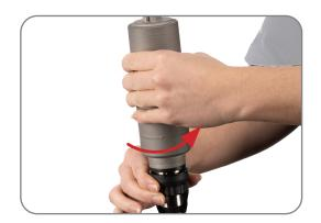
b. Remove the suppressor body from the barrel.
