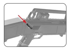
4. Remove the top cover by rotating it upward and lifting it off.
