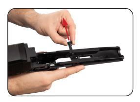
6. Ensure the grip is locked in position, then insert the FCU. Insert the back part first, then swing the front portion down into the chassis. The FCU fits tightly.
