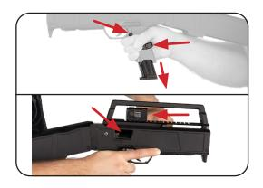
1. Reinsert the magazine. Push the magazine button without pushing the magazine grip release. The Magazine should stick out about 4 cm/1.5in being caught by the magazine grip release.
