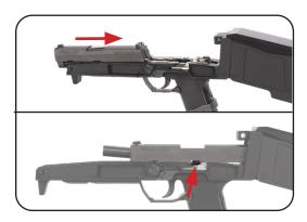
11. With the slide locked back, use a flat head screw driver to rotate the FCU retaining pin counterclockwise until it snaps in place, with the slot roughly vertical.
