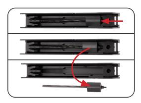
14. The spacer needs to be inserted with the horesshoe shaped protrusion pointing in the muzzle direction.
