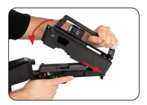
17. When the top cover is fully closed, push in the takedown pin until it is flush with the side of the top cover.
