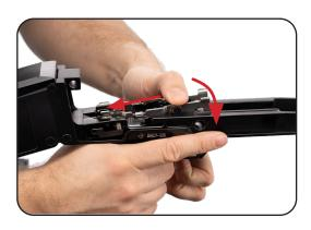
7. Ensure that the FCU is correctly seated in the chassis. The holes for the FCU retaining bolt need to line up with the corresponding holes in the chassis. The top of the FCU should only slightly protrude (~1/2mm) from the upper surface of the chassis.
