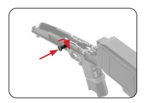
9. To install the barrel and slide, the FCU retaining pin must point to the 4 o'clock position.
