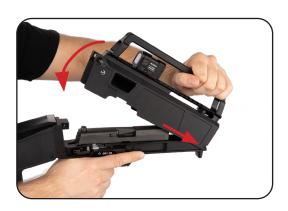
17. When the top cover is fully closed, push in the takedown pin until it is flush with the side of the top cover.
