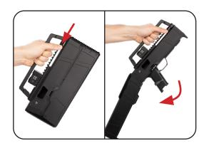
3. Push out the disassembly pin from the left to right. The pin is captured and will not detatch completly.
