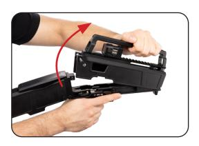
5. Push/Pull the FCU retaining pin out of the chassis.
