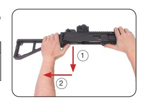
f. Pull the charging handle backwards until the recoil spring can be grasped, then pull the recoil spring backwards out of the lower receiver.
