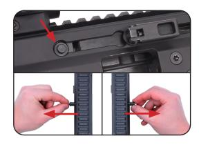
h. Pull the bolt rearward out of the receiver and remove it.
