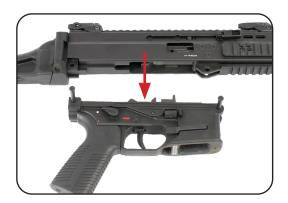
e. Grasp the stock, press it down and pull it back out of the upper receiver.
