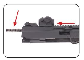
g. Pull the charging handle further back until the bolt securing pin is congruent with the cutout in the upper receiver.
