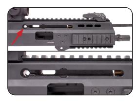
c. Make sure to insert the charging handle in the correct orientation in oder for the pin to slide into the recess in the charing handle carrier.
