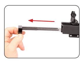
h. Pull the closing springs off the recoil spring plate.
