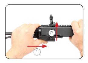
i. Connect the stock and the receiver by mounting the take-down pin.
