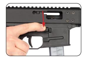
g. Slightly pull the bolt rearward until you can spot the brass of the chambered cartridge in order to verify the weapon is loaded.
