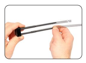
Pull the front charging handle back until it is aligned with the cutout in the receiver and pull out the front charging handle sideways
