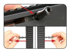
j. Pull the bolt rearward out of the receiver and remove it.
