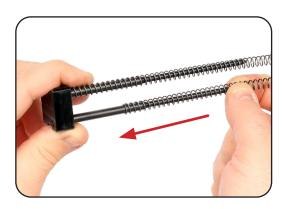
f. Insert the recoil spring plate with mounted recoil springs into the housing, making sure that the recoil springs are centered in the guide holes of the bolt.
