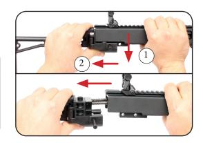
g. Pull the recoil spring plate and the closing springs backwards out of the housing.
