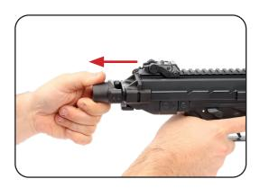
c. Pull out the stock until it reaches the desired position. Let the locking knob engage in the locking position.
