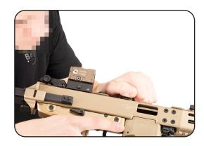
h. Rotate the fire selector to the "Decock" position in order to decock the weapon. The weapon is decocked if the green mark becomes visible on the left side.
