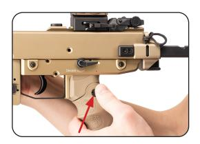
b. Fold the pistol grip until it reaches the end position.
