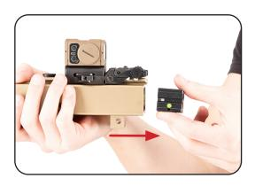
g. Remove charging handle through the port in the rearmost position.
