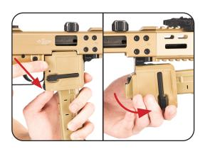
c. Push the magazine through the adapter until the stop.
