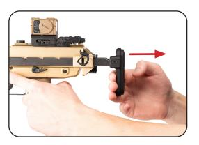
b. Pull out the stock with the non firing hand until it reaches the desired position.
