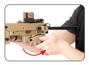
c. Grasp the weapon with one hand on the upper receiver, and fold the pistol grip out the stock until it snaps audibly in place.
