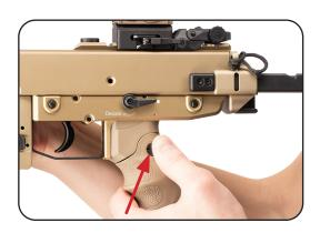
b. Fold the pistol grip until it reaches the end position.
