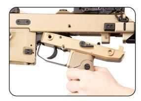
e. Grab stock assembly, pull it down and out of the upper receiver.
