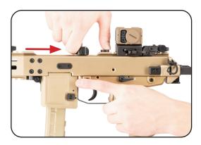
e. In order to close the bolt, pull back the charging handle until the bolt catch snaps out and allow the bolt to travel forward under its own power.
