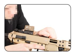
h. Rotate the fire selector to the "Decock" position in order to decock the weapon. The weapon is decocked if the green mark becomes visible on the left side.
