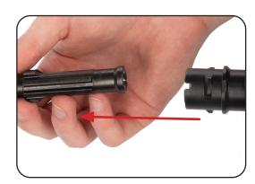
d. Pull and separate the recoil spring and guide rod from the top cover.
