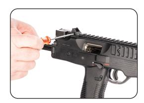
b. One full turn of the sight adjustment screw in a clockwise direction changes the point of impact to the left therefore turn in the clockwise direction when the point of impact is right off.
