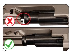
p. Rotate the barrel guide upwards that the side surfaces align with the bolt.
