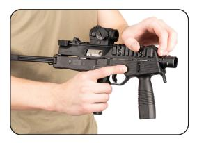
f. With light pressure push the bolt and barrel assembly to the rear of the top cover and lift them out.
