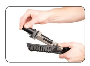
g. Hold barrel assembly and slowly separate from the bolt, until barrel and bolt are in two pieces.
