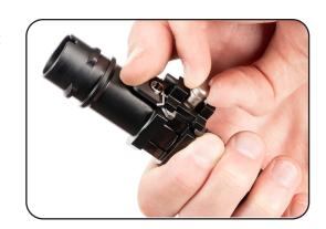
c. Draw the barrel forward from the barrel guide.
