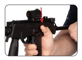
g. Slightly pull the bolt rearward until you can spot the brass of the chambered cartridge in order to verify the weapon is loaded.
