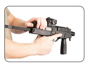
e. Press the detent plate and remove top cover with barrel assembly upward in a straight movement.
