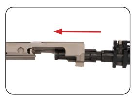
o. Push the barrel into the bolt all the way to the stop until the barrel and bolt face are in contact.
