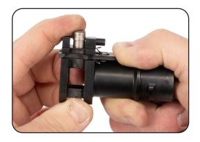
o. Insert the barrel into the front of barrel guide.
