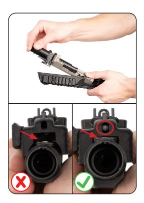
r. Check hammer to be cocked and locking sear to be in left position. If hammer or sear are in wrong position, push into correct.
