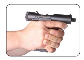
d. Extract the spent case by rotating the breech operating handle 90° counterclockwise and pulling the bolt with a swift motion rearwards to the fully open position while tilting the weapon at least 90 degrees to one side, allowing the extracted case to fall out of the weapon.
