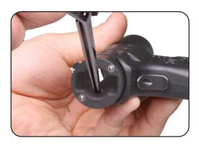
d. Align the groove in the bolt with the pin in the trigger safety and insert the bolt into the housing.
