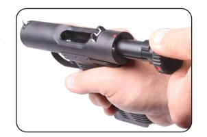
e. Load the next cartridge by pushing the breech in one fluent motion to fully closed position and rotating the bolt operating handle 90° clockwise until the red marks fit.
