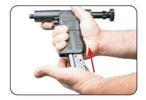
d. Push the bolt operating handle in one fluent motion to fully closed position and rotate the bolt operating handle 90° clockwise until the red marks align.
