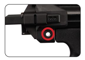
d. Install the takedown pin (two pins are present on the MP5K) with the spring in front. Push the takedown pin through the receiver until the spring comes out on the opposite side and locks the stock.
