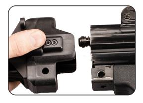
c. Insert the stock into the receiver as far as it will go. The hole of the receiver and the stock must be concentrically superimposed.
