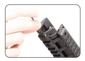
b. Plug the back of the handguard into the receiver.
