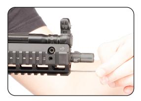
b. Loosen the hexagon socket head cap screw.
